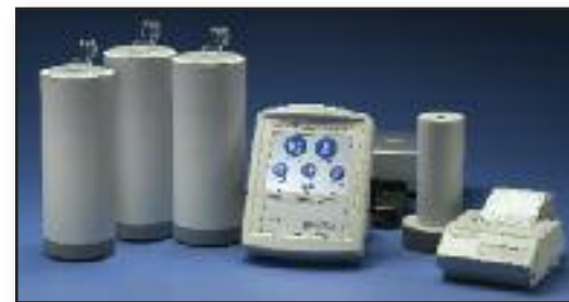
◀ Atomlab 500Plus with additional chambers and wipe test counter.
